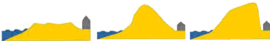
Figure 4. Illustration of dune base shapes (from left to right: eroded, triangular and trapezoid) (© ONF).
