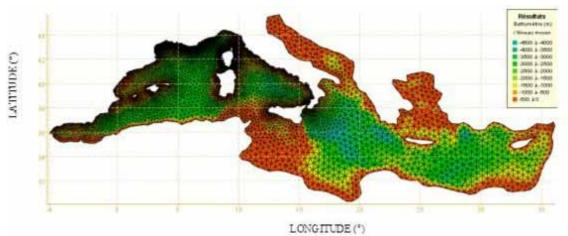
Figure 1. Computational mesh used for the wave simulations with TOMAWAC.
