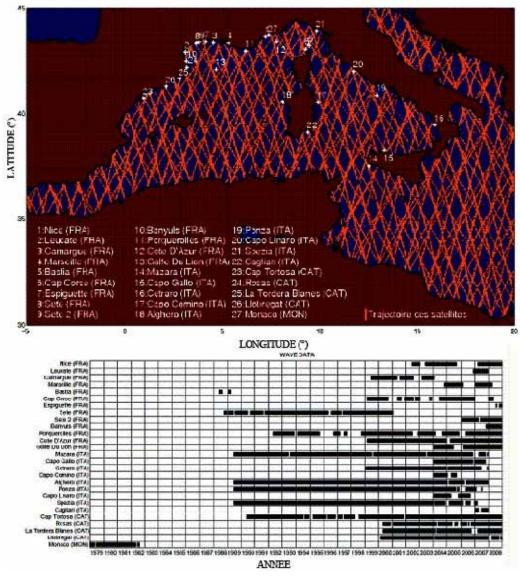
Figure 2. Top : Wave Buoy positions and ground track of satellites; bottom: Periods of measurement of wave buoys used for comparison.
