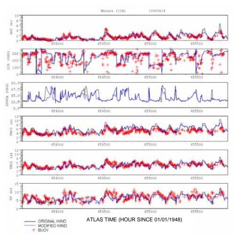
Figure 3. Comparison of model results with buoy data of Mazara for the last quarter of 1999.
