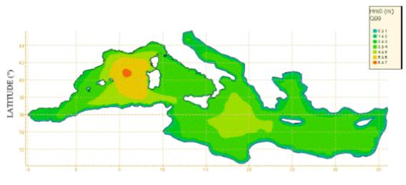
**LONGITUDE** (\*) Figure 8. Chart of the Q99 of wave height H<sub>mo</sub> computed over the period 1979-2008.
