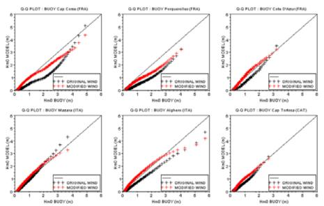
Figure 5. Q-Q (Q1-Q99) plot between measurements and model for 6 buoys.
