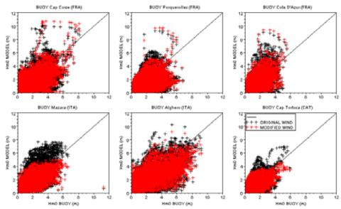
Figure 4. Distribution of  $H_{mo}$  between measurements and model for 6 buoys.
