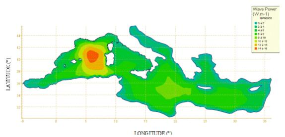
Figure 7. Chart of the mean wave power computed over the period 1979-2008.
