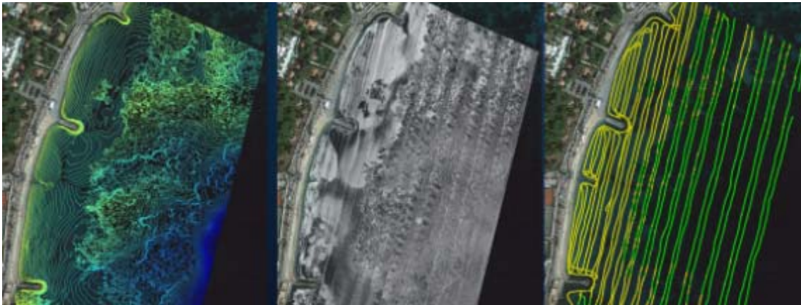
Figure 5. Various layers of information, from left to right: bathymetry, side scan sonar imagery and AGDS classification.
