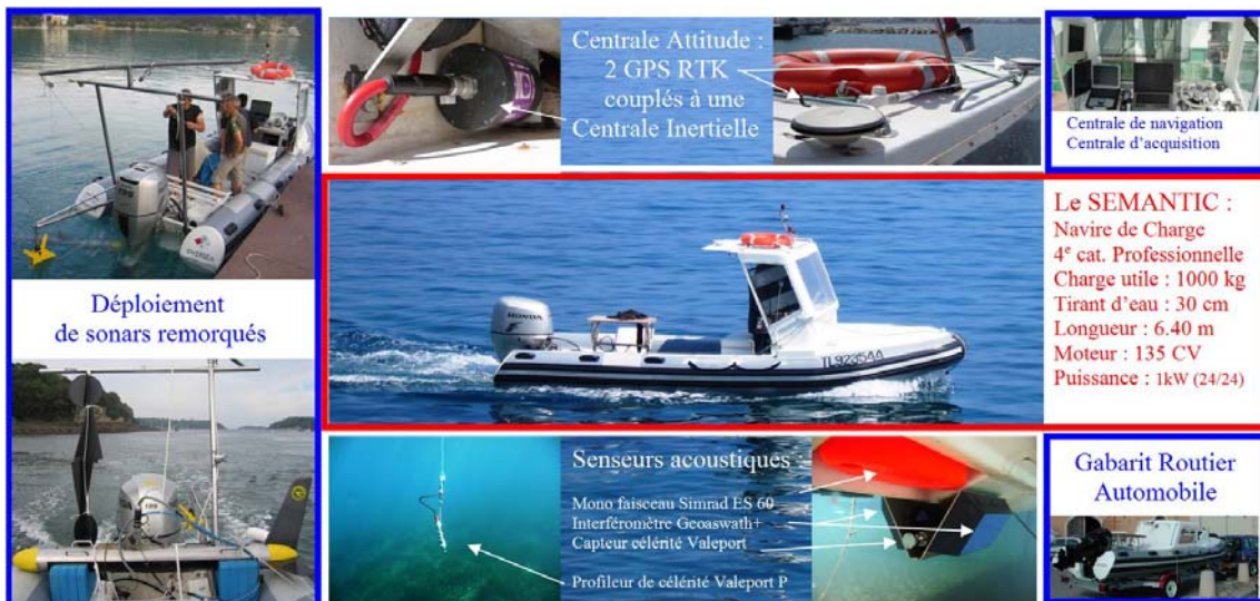
Figure 2. Fully instrumented oceanographic ship (comments are in French).
